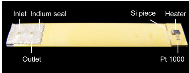
Figure 5.3: Single-stage microcooler with a silicon piece, a heater and a temperature sensor.
